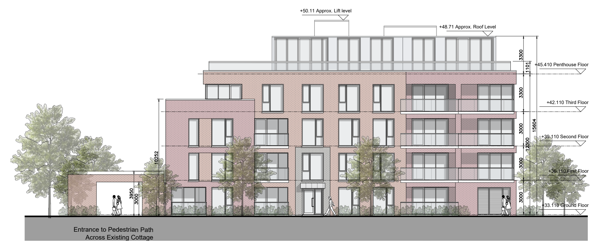
APARTMENT BLOCK C SOUTH ELEVATION (STREET ELEVATION)
